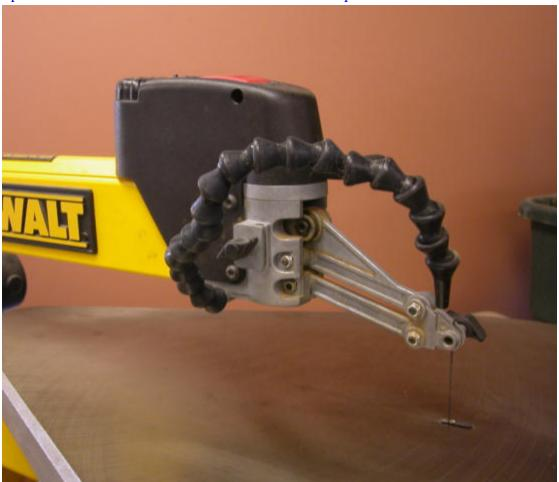
frame. I moved the entire assembly out away from the yellow frame nearly 1/8" and temporarily clamped it in place. I ran the saw slow and the blade travel was nearly PERFECT!
