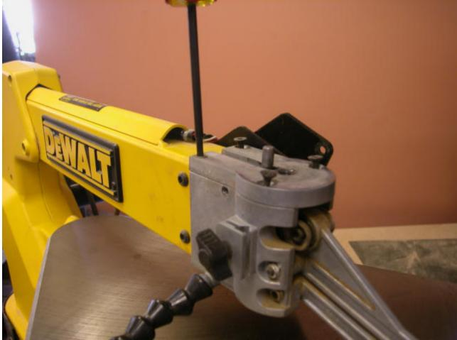
putting a metal ruler or something behind the blade and turning the motor by hand to see the difference. had a request from Rick for a picture of what I moved to achieve near zero forward blade travel. It's a bit blurry since my good camera is hiding from me and I had to use an old cheapy. It should give an idea on how much I moved it. You can see the new gap between the lower blade assembly and
